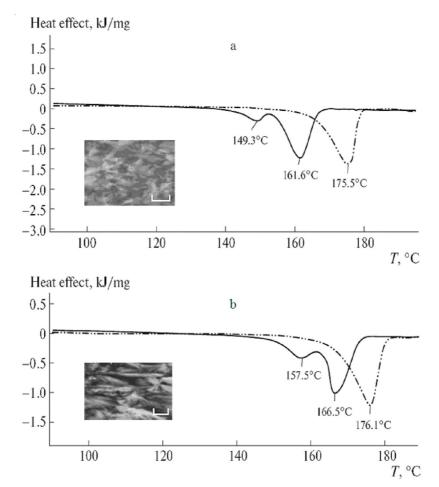
Fig. 2. Thermograms of melting of the fibrous matrix of PHB (a) before and (b) after mechanical treatment via rolling: The single maximum to the right is related to the first temperature scan; the binary maximum corresponds to the second temperature scan. Inserts: SEM images of crystalline regions of PHBs in the form of (a) a fibrous matrix and (b) a fibrous matrix after cold rolling. The markers indicate 0.2 μm
