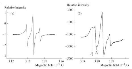
Fig. 3. ESR spectra of TEMPO in (a) the PHB film and (b) the fibrous matrix at 25 °C that demonstrate the superposition of two simple spectra of radicals with different correlation times (rapid and slow modes)
