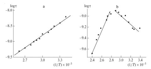
Fig. 4. Dependences of correlation time on inverse temperature for (a) the fibrous matrix and (b) the same matrix after cold rolling
