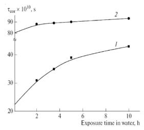
Fig. 5. Correlation time vs. time of contact with the aqueous medium: (1) pristine fibrous matrix and (2) the same matrix after mechanical treatment
