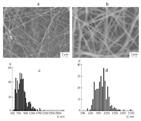
Fig. 1. (a, b) SEM images of PHB fibers prepared via electrospinning of (a) 5 and (b) 7 % polymer solutions; (c, d) the corresponding fiber-diameter distributions
