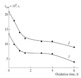
Fig. 6. Correlation time of TEMPO vs. time of ozone oxidation in (1) the pristine fibrous matrix and (2) in the same matrix after cold rolling
